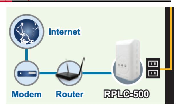
Connecting to PC / Smart TV / NB / Blu-ray Player / Media Player / IP Phone: Insert One end of the RJ45 Cable (Recommend using Cat 5E cable or above) to this port, and the other end to the other devices. Then plug into the electrical outlet.
